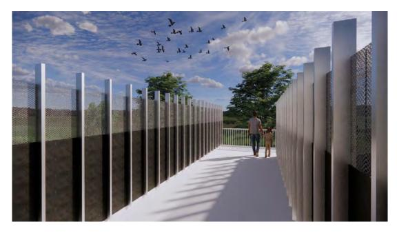
Figure 4-48 3D image of parapet heightening solution for footbridges
