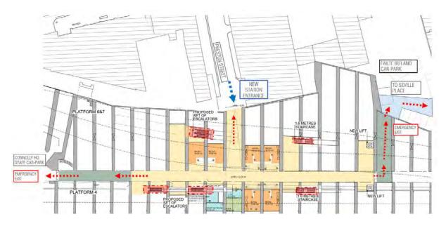
Figure 4-63 Plan view of the proposed layout within the Connolly Station vaults
