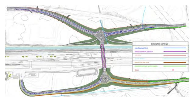
Figure 4-233 L5041 Drainage system proposed for each alignment
