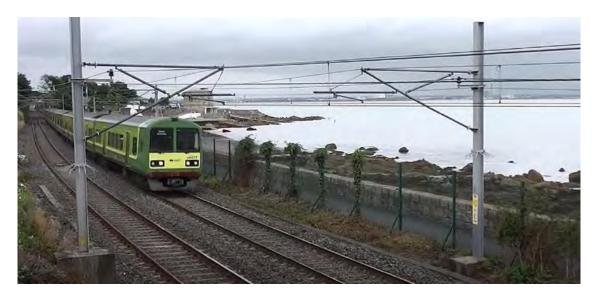
Figure 4-23 Current DART cantilever layout
